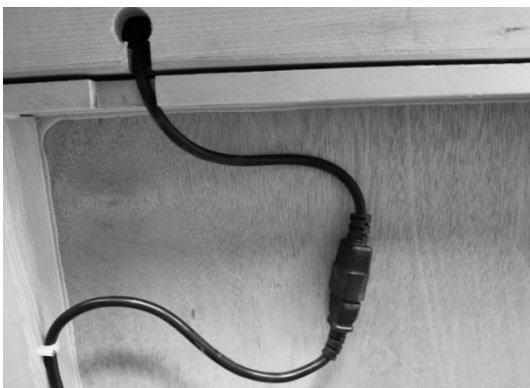
(1) Plug in the connectors of heater cables, make sure the cables not pinched between
