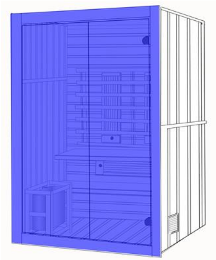
(9) install Front panel to Left panel and Right panel with preset outside buckles.
